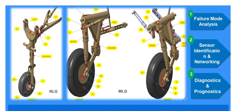
Sensing ex: Tire pressure, Drag, Side & Vertical Load, Brake Temperature, Brake pressure
